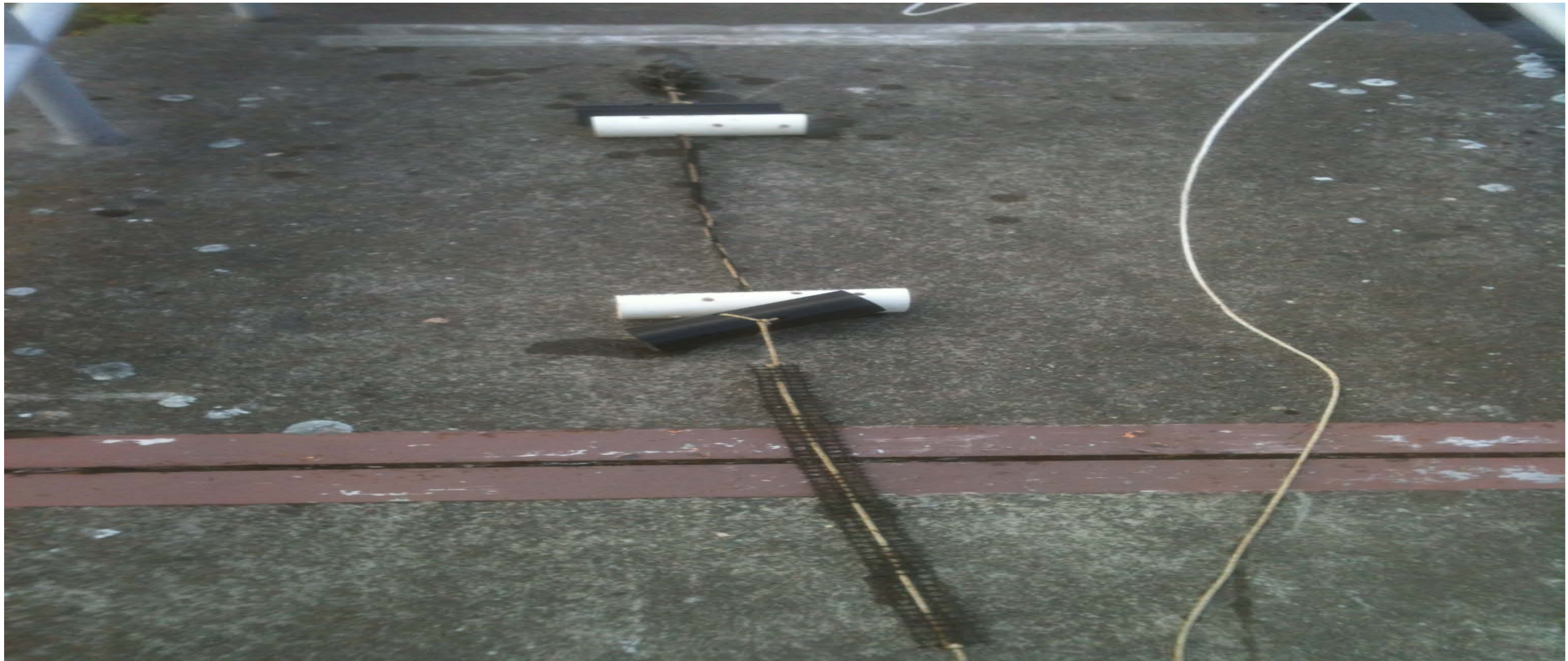
Updated and newly deployed dreissenid mussels traps installed at both adult ladder count stations
